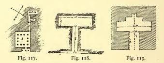
sometimes it is recessed just opposite the entrance passage, and then the plan forms a cross, of which the head is longer or shorter (fig. 119). This was the ordinary arrangement, but the architect was free to reject it, if he so pleased. Here, a chapel consists of two parallel lobbies connected by a cross passage
